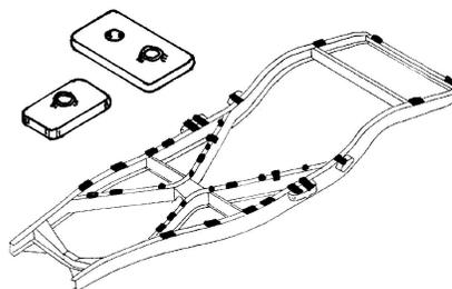
1932-47 Pickups used a heavy wood body to frame spacer block. The proper shape and spacing are important for proper body to fender and hood alignment.
