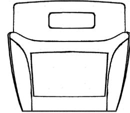
One door hangs out at the bottom, and the opposite is in at the bottom. Note this should be checked with the doors unlatched. Correct by shimming the body counterclockwise, or the cowl clockwise. Opposite on suicide door cars.
