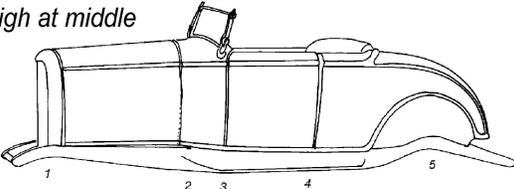
Wide gap at top of door tapering to normal at bottom.
