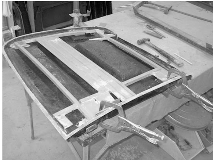
Steel installation inside a '34 roadster door
