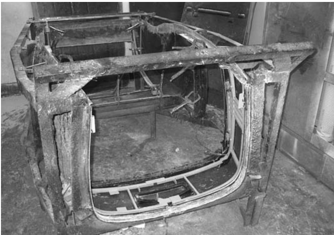
Steel installation in the cowl section of a '32 roadster
